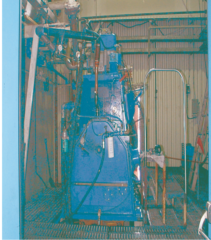
Figure 1: SCRE-251 test engine
